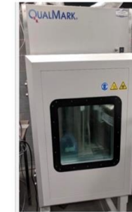
High Accelerated Life Test with shock vibration
