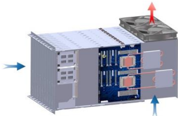
Loop Heat Pipe 1 Li et al. (2021)
