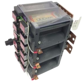
SiC inverter with air cooled heat sink
